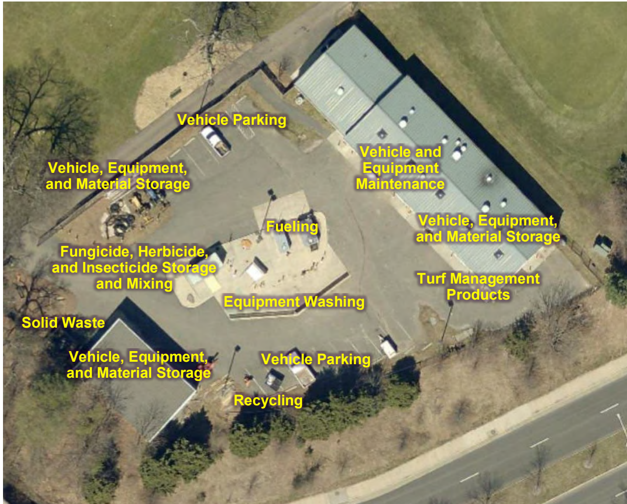
Figure 3A – Maintenance Facility Potential Pollutant Sources
