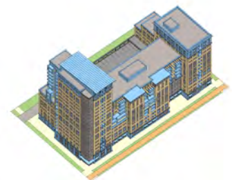
4 - Articulate the building by establishing bays, applying building elements, changing materials, etc.
