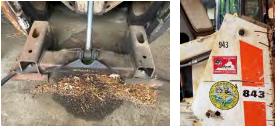
Leaking hydraulic fluid from Truck 879.
