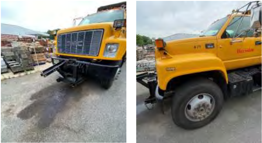
Leaking hydraulic fluid from Truck 879.
