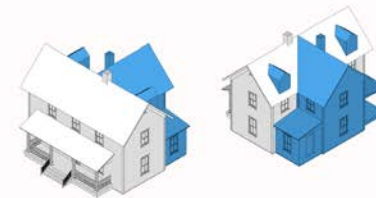
2-story residential - appropriate rear & dormer additions
