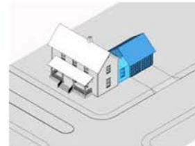
Garage (dark blue) located behind the principle building, connected by an architectural hyphen (light blue)
