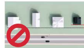
A new building, to the right, inappropriately set back from the existing buildings along the block
