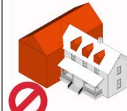
2-story residential - inappropriate rear & dormer additions
