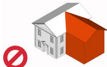
Commercial 2-story - inappropriate rear addition
