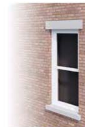
Brick lintel and sill made of stone, cast stone, concrete, or wood. Lintels should extend at least 4" beyond the edge of the masonry opening.
