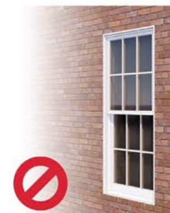
Flush Framing - Not Recommended
