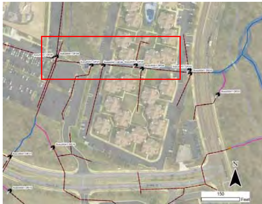
Figure 3: Inaccessible outfalls underneath Residence Inn complex. Outfalls outlined in red.
