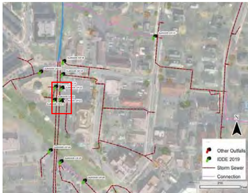
Figure 4: Inaccessible outfalls underneath Center Street/Herndon Fortnightly Library. Outfalls outlined in red.
