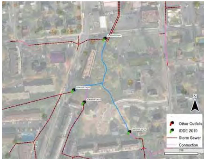
Figure 5: Outfall 09.OF03 was determined to convey piped stream flow. Outfall OF02 will be adjusted to reflect drainage from curb inlet.
