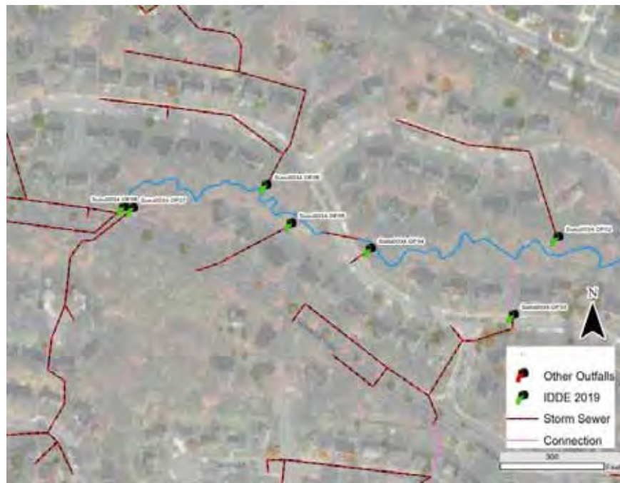
Figure 6: Outfalls 34.OF08 and 34.OF03 convey piped stream flow.
